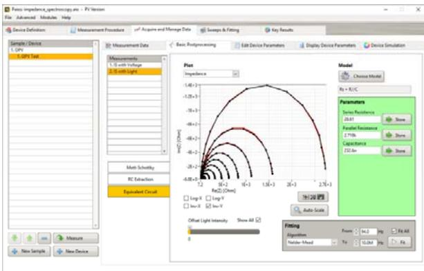
The most popular way to analyze impedance spectroscopy data is equivalent circuit fitting. Paios has integrated a routine for such fits.
