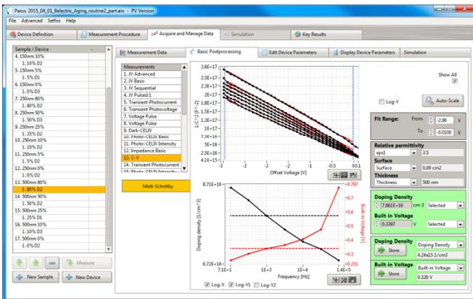
With a Mott-Schottky analysis the doping density of a semiconductor can be extracted from CV measurements (provided the device is thick enough).
