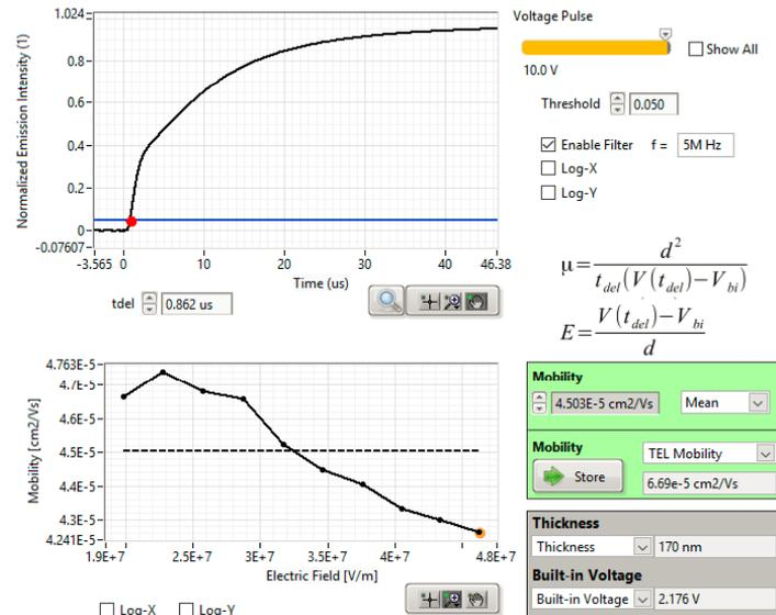
From the electroluminescence decay after voltage turn-off the luminescence lifetime of the emitter can be extracted.
