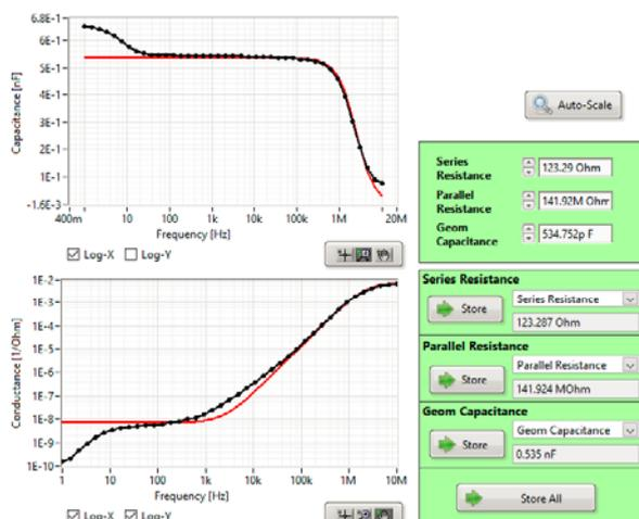
A very reliable method to extract the series resistance and the geometric capacitance from impedance spectroscopy data
