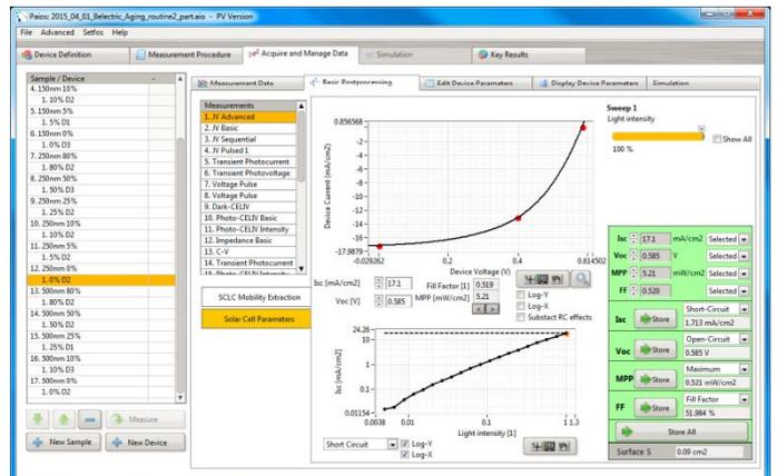
Extract the parameters of the one-diode model for solar cells: ideality factor, dark saturation current, series resistance and parallel resistance.
