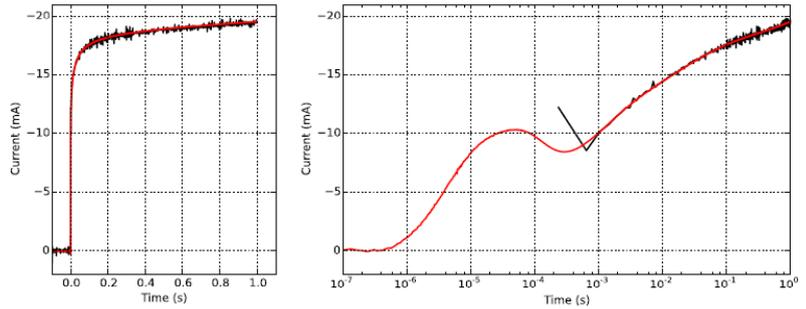
Transient photocurrent of a perovskite solar cell with linear time scale (left) and logarithmic time scale (right).
