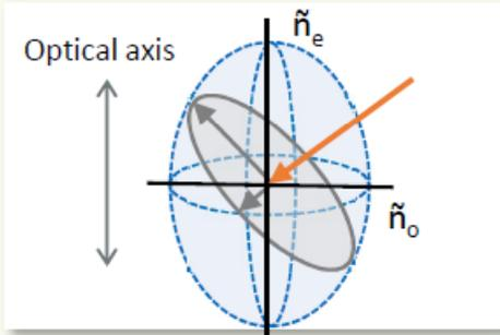
Determine the emitter orientation in a birefringent emitting layer
