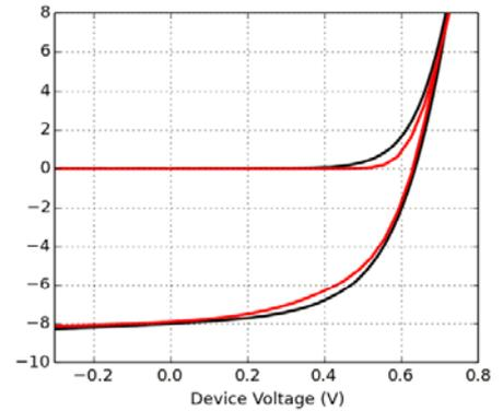
IV-curve simulation (illuminated and dark) after fitting.
