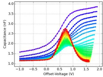
Capacitance-Voltage curves of an organic solar cell at different degradation stages.
