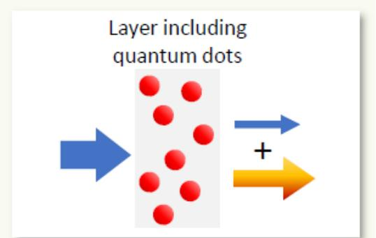
Analyze the effect of incorporating quantum dots in a color conversion film
