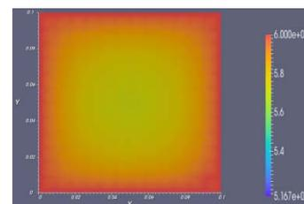
OLED with a metal grid leading to more uniform potential
